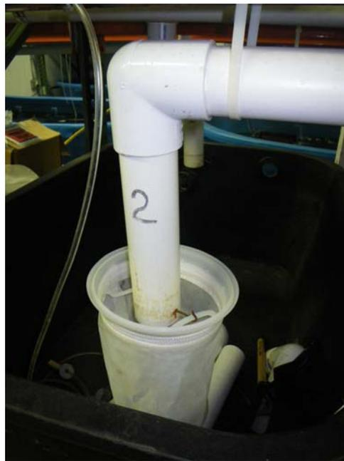
**Figure 13.** Overflow from host fish tank with filter to collect juvenile mussels.
