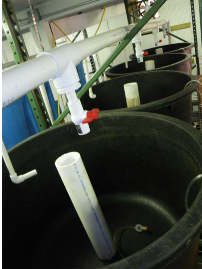
**Figure 12.** Holding tanks for infested host fishes with double stand pipe to continuously draw transformed juvenile mussels out with overflow.
